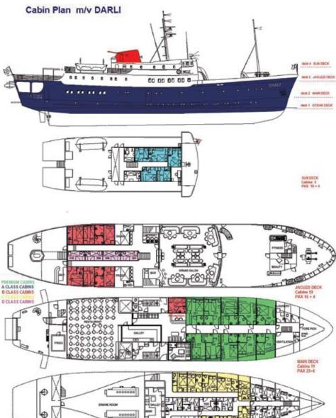
57,50 m 11,00 m Croatian / CRO 1960. Stord / Norway according DNV Rebuilt and totaly refit Tonnage GT Max speed 2006. Rijeka /Cróatia 995 t 12 kn
