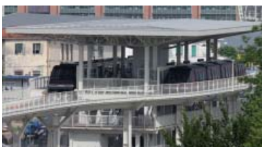
Two trains on a single guideway bypassing each other at an intermediate station
