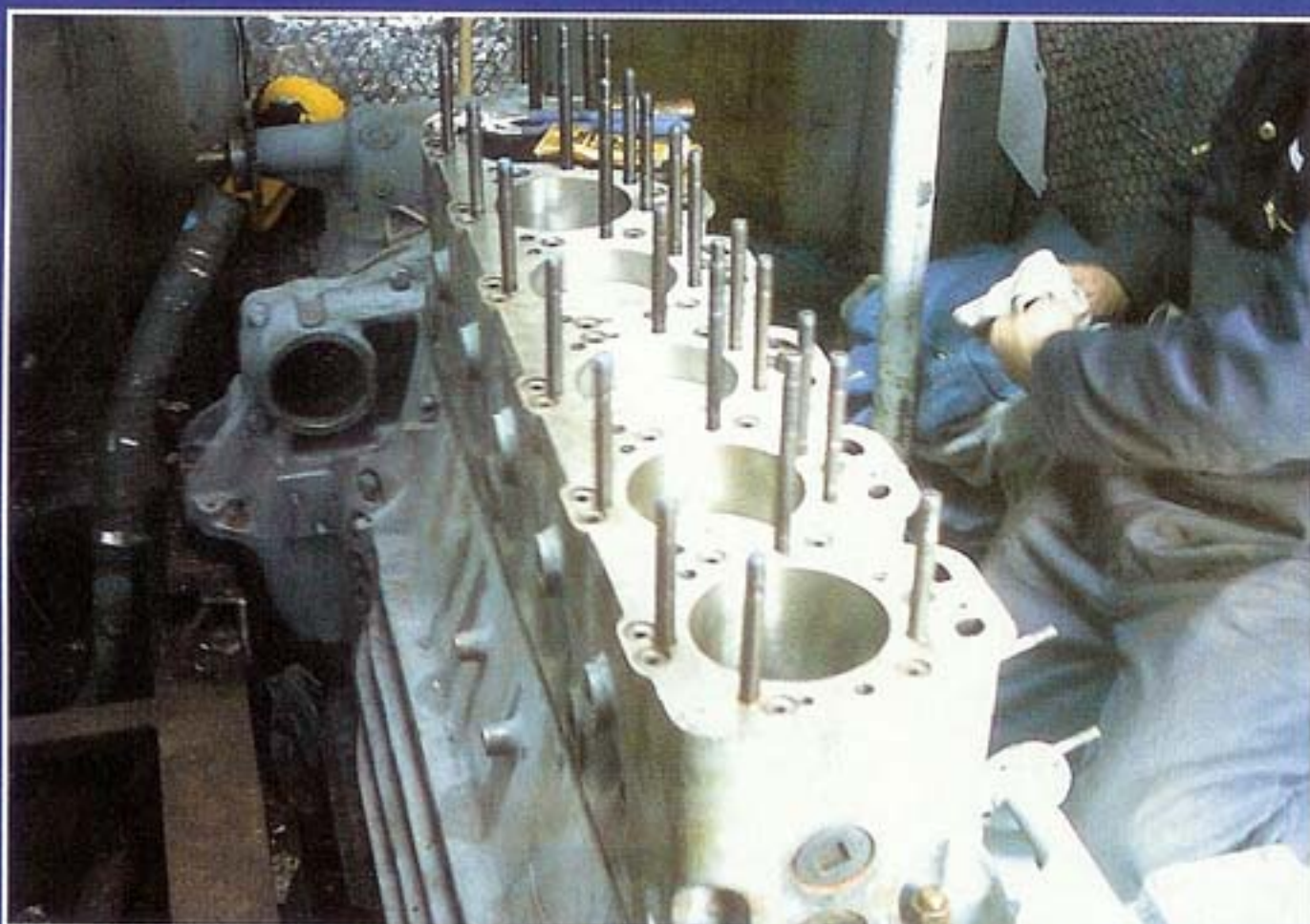
Rebuild of the Gardner 6LX unit – probably the oldest example in regular daily use.
