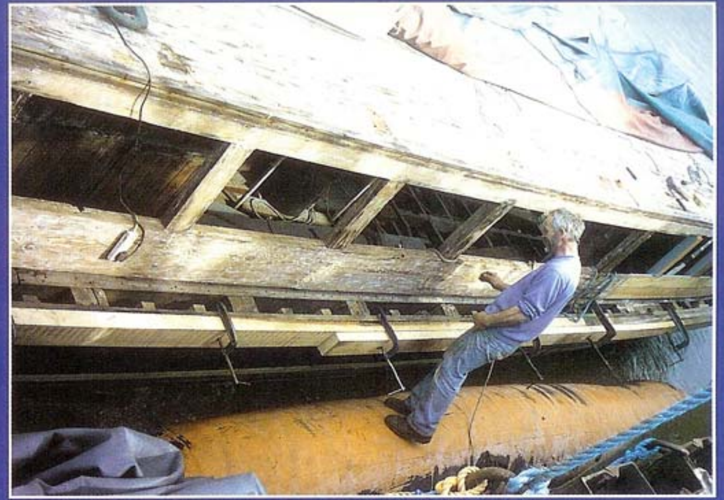
Repairing the cabin sides.
